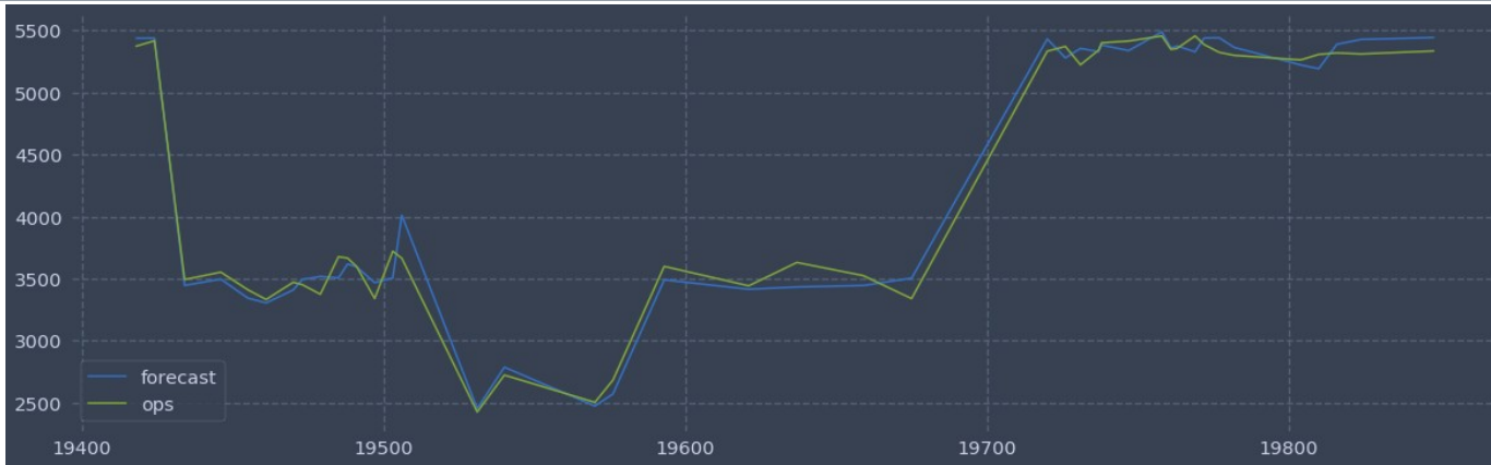
Forecast of a Memory Workload's performance over time for a single container vs actual operations per second
